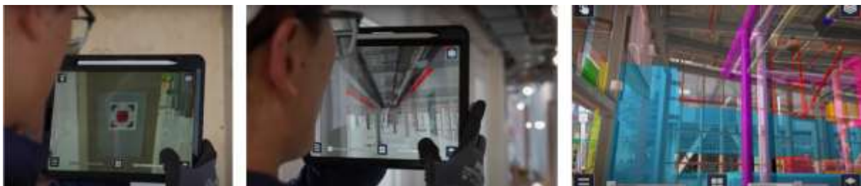
Fig. 1 – AR technology allows you to visualize a 3D model of an object through a tablet camera
