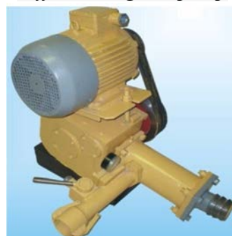
Grout pump of angle pump column
