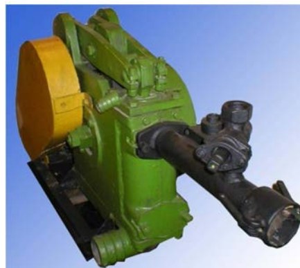
Differential grout pump
