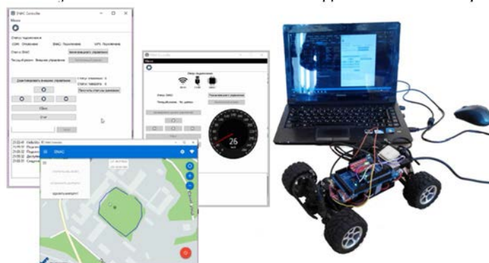
Device model of road marking with the satellite radio navigation orientation system
