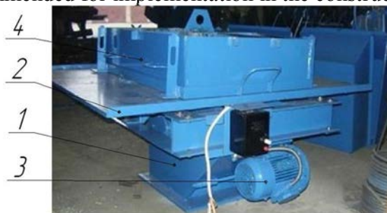
1 – fixed section; 2 – movable frame; 3 – electric motor; 4 – moulding box UA-6 Shock-and-vibration machine
