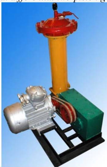
Single-piston grout pump with combined surge dampener
